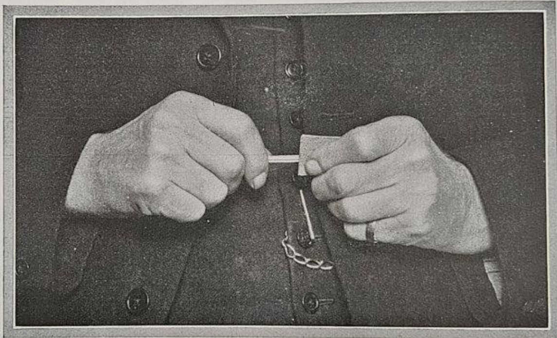
Fig. 8. METHOD OF IGNITING ONE OF WALKER'S FRICTION-LIGHTS BY DRAWING IT BETWEEN FOLDED SAND-PAPER TIGHTLY NIPPED.
